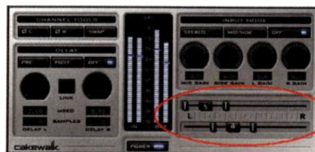
Fig. 2. Sonar's Channel Tools plug-in includes sliders that allow adjusting the angle and width of a stereo signal's left and right channels independently.
